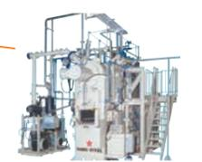
**Vacuum carburizing furnace "SyncroTherm"**
