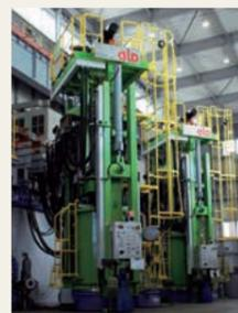
Vacuum arc remelting (VAR) furnaces at Shibukawa Plant
