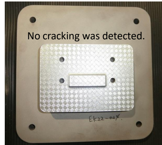
Fig. 4 Appearance of the 3D-printed test mold
