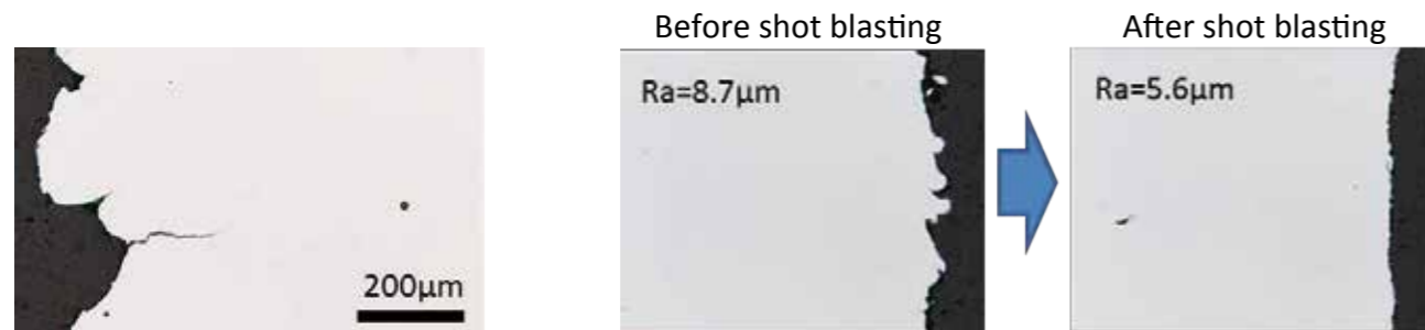
Fig. 12 Initial cracks caused by tempering after 3D printing.
