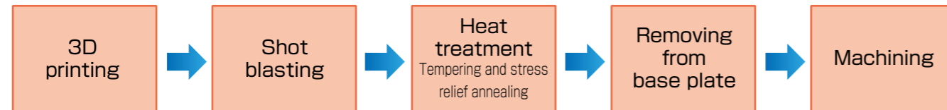
Fig. 11 Typical mold manufacturing process using AMDAP™ HTC.
