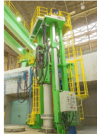
A VAR furnace installed at Chita Second Plant
